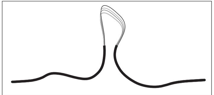
4. Use a wire tie to keep the wire loop intact and act as a strain relief.
