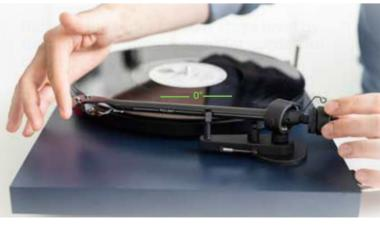
(not the whole weight) so the '0' is in line with marker at the back of the tonearm.
