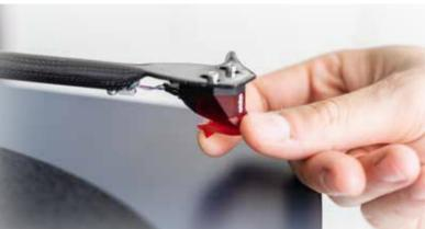
Remove the needle protection cover.
